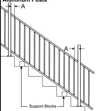
Use Avant Aluminum Adjustable Panel to determine the angle of stair installation. To do this, use support blocks resting on the stair tread. Position support blocks so that the position of the bottom rail meets the spacing requirement of your building code.
