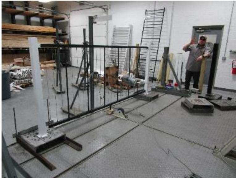
Photo No. 1 In-Fill Load Test at Center of Vertical Cable
