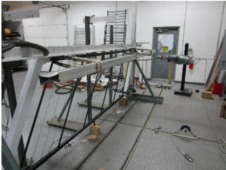
Photo No. 4 Concentrated Load Test at Ends of Top Rail (Brackets)
