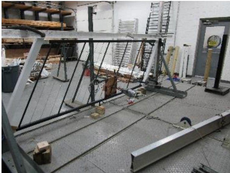
Photo No. 2 In-Fill Load Test at Bottom of Intermediate Support Baluster
