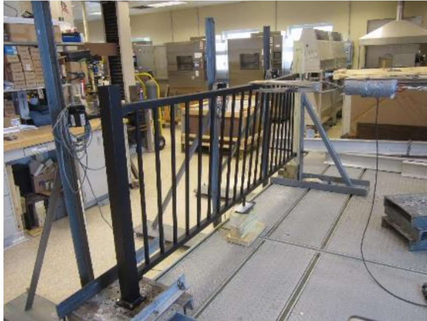
Photo No. 5 Concentrated Load Test at Mid-Span of Top Rail
