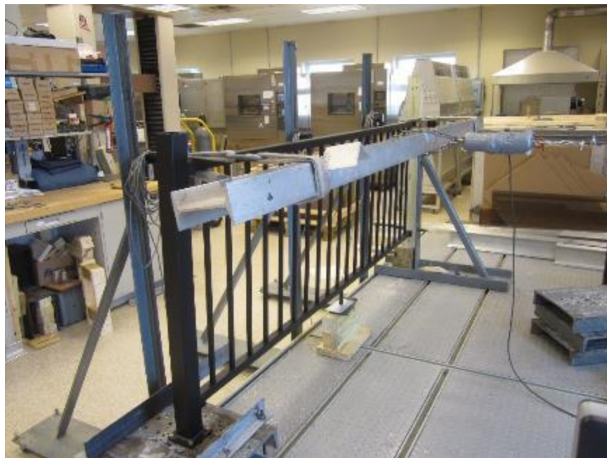
Photo No. 6 Concentrated Load Test at Ends of Top Rail
