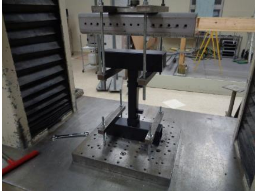
Photo No. 1 Assembly Fastener Test Setup (Aluminum Post)
