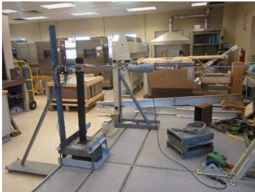
Photo No. 7 Concentrated Load Test at Top of Post Mount
