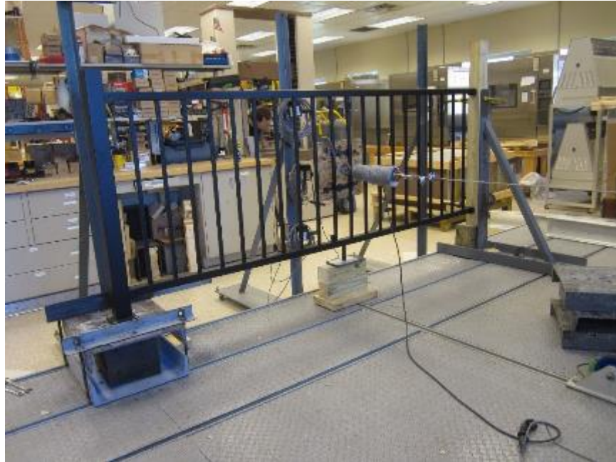
Photo No. 3 In-Fill Load Test at Center of Two Pickets
